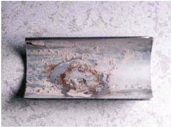
Figure 2 Pitting Under Scale in Stainless Steel Tube (Photo Courtesy of Howell Image Sciences)
