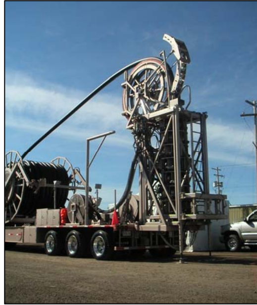
Roller Reduction Unit (RRU) – Progressively reduces the plastic liner OD through a series of precision sized roller banks.
